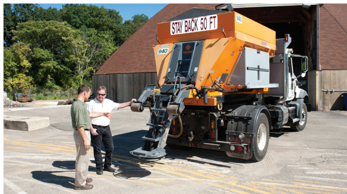
Chuck Novak (left), Street and Sanitation Commissioner for the City of Cuyahoga Falls, Ohio, and Dave Johnson, Sales Manager for Bell Equipment, Novak's local Epoke representative, discuss the material pre-wetting capabilities of an Epoke bulk spreader. By adding brine to dry salt, the city optimally controls its salt spend – and just how accurately dispensed material coats targeted lanes.
