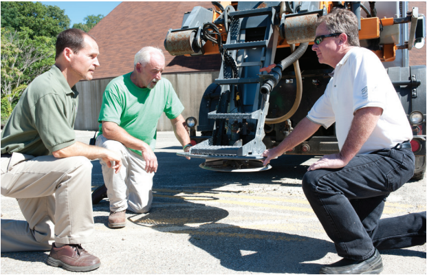
Chuck Novak, Street and Sanitation Commissioner for the City of Cuyahoga Falls; Ron Garberoglio, one of the city’s Heavy Equipment Operators; and Dave Johnson, Novak’s local Epoke rep, examine the spreader disk on an Epoke 4400 bulk spreader. Novak especially likes the way the driver, by simply turning a knob inside the cab, can easily adjust just how much material can be put down per lane.
